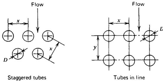
Fig. 45.35 Pressure drop factors for flow of air or flue gas through tube banks.<sup>1</sup>
