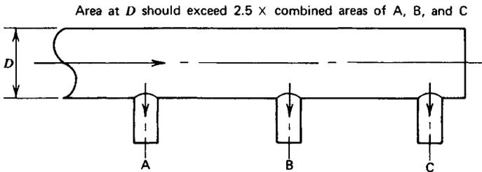
Fig. 45.34 Pressure drop in velocity heads for flow of air or flue gas through orifices, elbows, and lateral outlets.<sup>1</sup>
