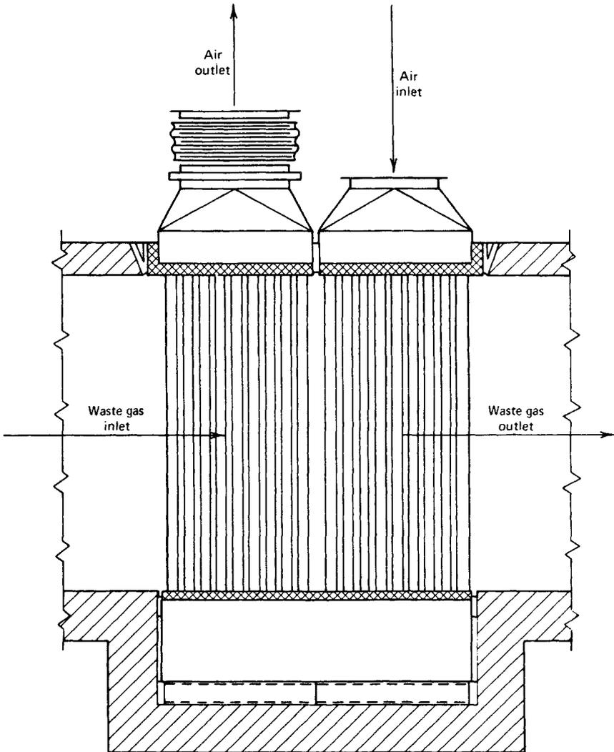
Fig. 45.46 Cross-flow-type recuperator in waste-gas flue.<sup>1</sup> (Courtesy Thermal Transfer Corporation.)
