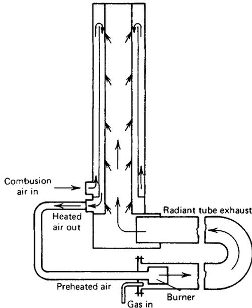
**Fig. 45.48** Radiant tube recuperator.<sup>1</sup> (Courtesy Holcroft Division, Thermo-Electron Corp.)
