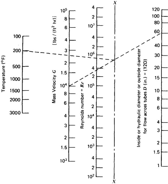
Fig. 45.36 Reynolds number ( $Re$ ) for flow of air or flue gas through tubes or across tube banks.<sup>1</sup>
