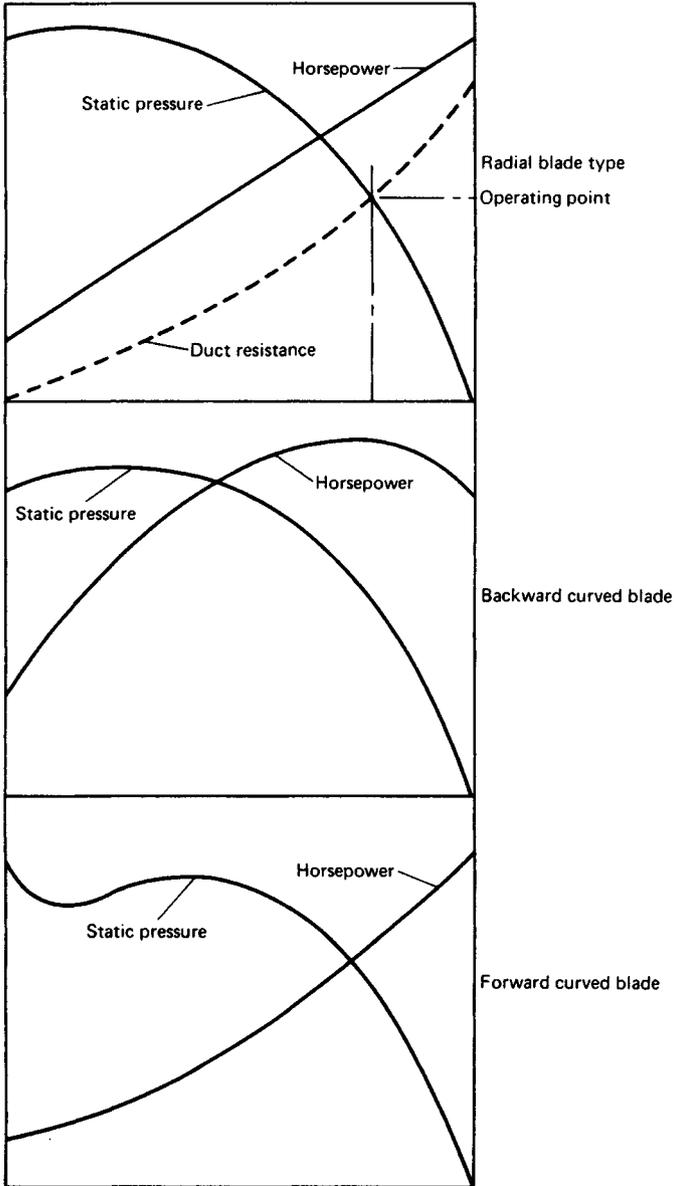
Fig. 45.39 Centrifugal fan characteristics.<sup>1</sup>
