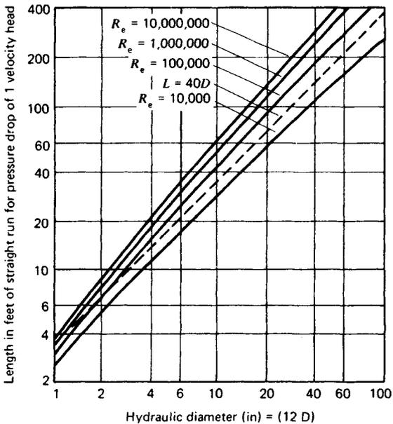
Fig. 45.37 Length in feet for pressure drop of one velocity head, for flow of air or flue gas, as a function of  $Re$  and  $D$ .<sup>1</sup>
