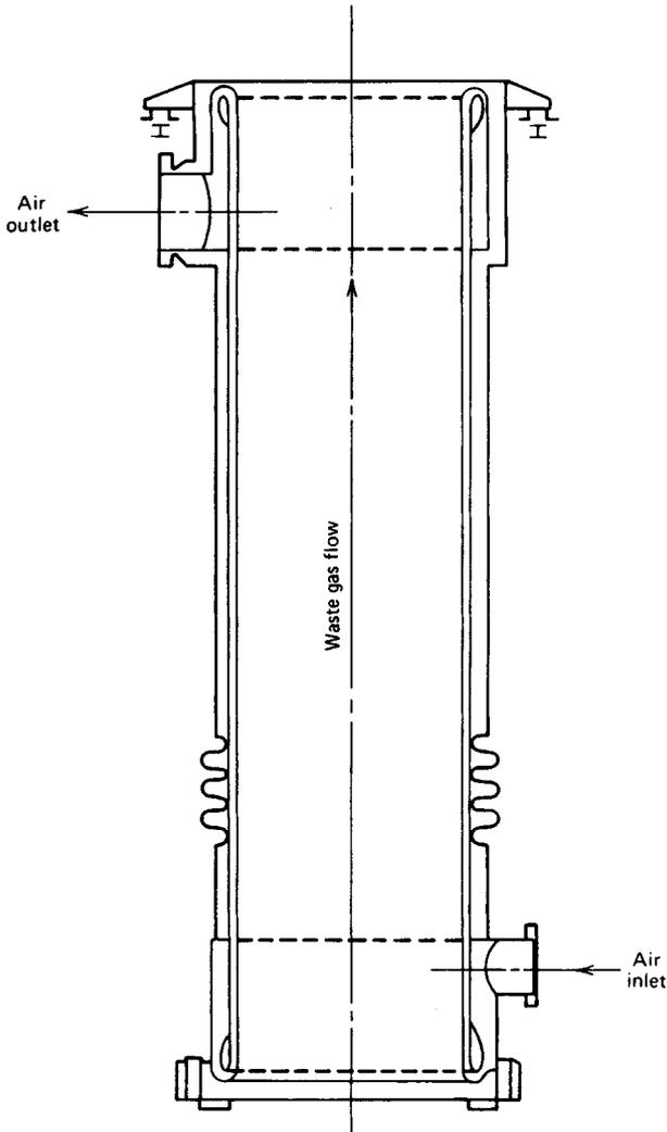
Fig. 45.45 Stack-type recuperator.<sup>1</sup> (Courtesy Morgan Engineering Company.)
