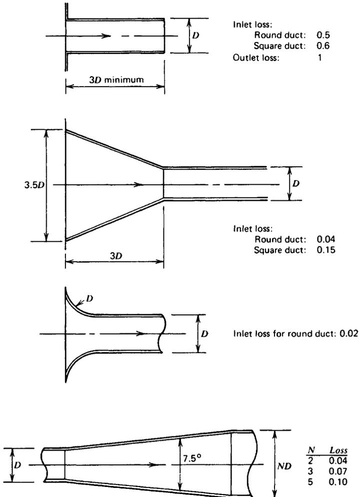
Fig. 45.33 Pressure drop in velocity heads for flow of air or flue gas through entrance configurations or expansion sections.<sup>1</sup>
