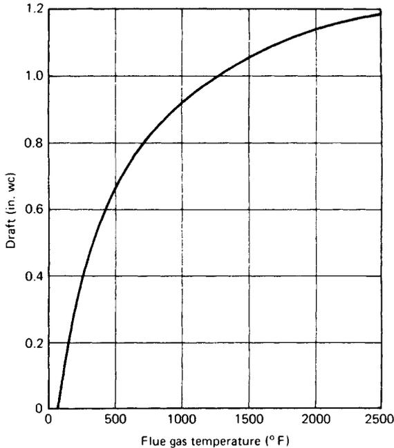
Fig. 45.38 Stack draft for ambient  $T_g = 70^\circ\text{F}$  and  $\text{psia} = 14.7 \text{ lb/in.}^2$ .
