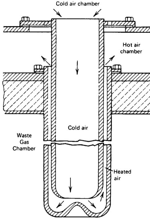
**Fig. 45.47** Concentric tube recuperator, Hazen type.<sup>1</sup> (Courtesy C-E Air Preheater Division, Combustion Engineering, Inc.)
