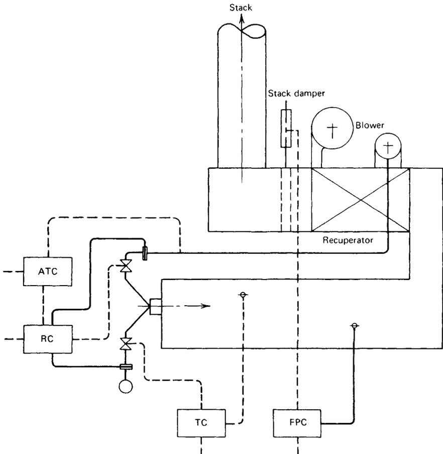
Fig. 45.43 Combustion control diagram for recuperative furnace.<sup>1</sup>
