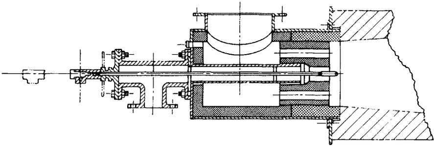
**Fig. 45.42** Dual fuel burner with removable oil nozzle.<sup>1</sup> (Courtesy Bloom Engineering Company.)
