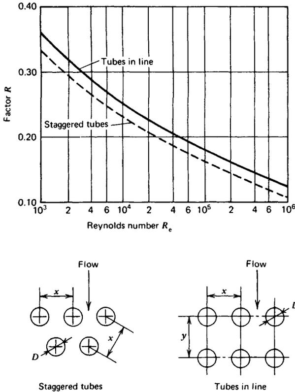
Fig. 45.32 Heat loss for flow of air or flue gas across tube banks at atmospheric pressure (velocity head)  $\times F \times R$ .
