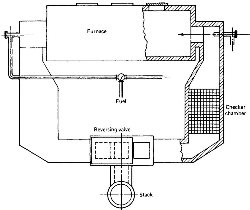
Fig. 45.44 Regenerative furnace diagram.<sup>1</sup>
