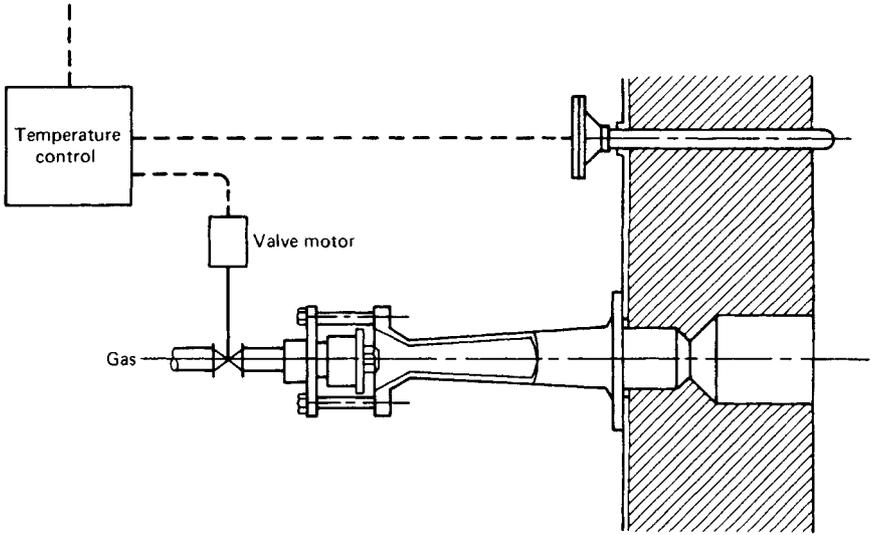
Fig. 45.40 Air/gas ratio control by high-pressure gas inspirator.<sup>1</sup>
