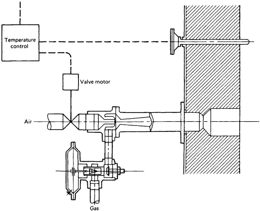
Fig. 45.41 Air/gas ratio control by air inspirator.<sup>1</sup>
